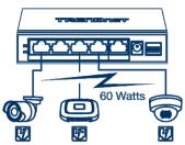
A 60W PoE power budget supplies up to four Power over Ethernet devices.
