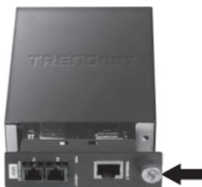
3. Slide the media converter into an available slot and fasten the thumbscrew.
