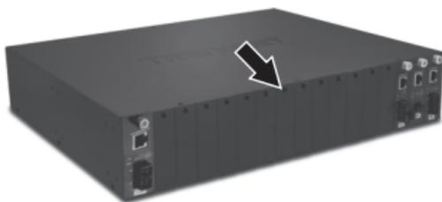
2. Unfasten the thumbscrew and remove the fiber converter from the metal casing.
