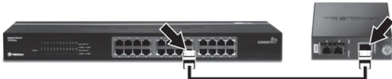
2. Connect the fiber cable to the fiber converters.
