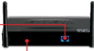
2. Connect the AC Power Adapter to the TEW-670AP and then to a power outlet.
