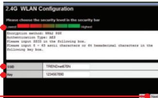
6. Enter the desired SSID and Key. Then click Next. By default, the SSID for 2.4G WLAN is TRENDnet670N.
