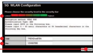
8. Enter the desired SSID and Key. Then click Next. (By default, the SSID for 5GHz WLAN is TRENDnet670A).
