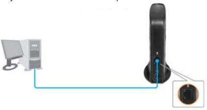
2. Plug in the power adapter and verify the Power & Ethernet LEDs are light.
