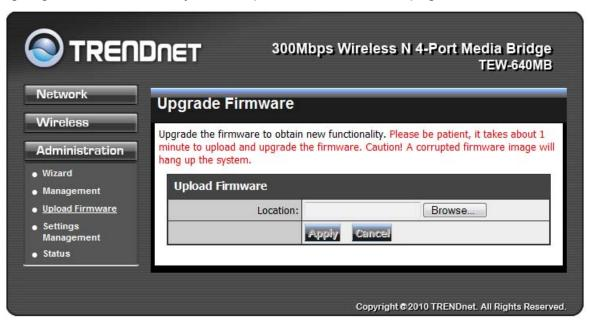
Once you have a firmware saved on your computer, use this option upload the firmware. Click on **Browse** and select the firmware file, then click **Apply** to upload the file into the adapter.
