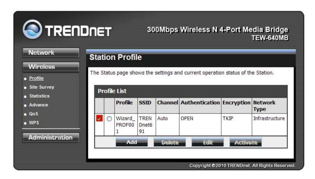
Configure the setting to connect to a wireless network, selection option for network type, SSID, and wireless security. The profile can be edited, deleted and made active from this option. There are several ways to connect to your wireless network, go through the setup wizard, add a new profile or search using site survey feature.
