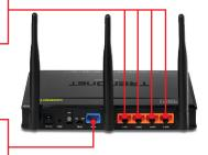
Connect one end of a network cable to the TEW-639GR's WAN port. Connect the other end of the cable to your modem's network port.
