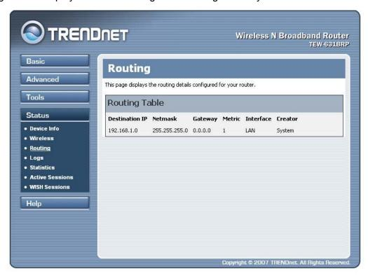
A value of 0.0.0.0 for gateway means there is no next hop, and the IP address is directly connected to the router on the interface specified: LAN or WAN. A value of 0.0.0.0 in both the destination IP and netmask means that this is the default route.
