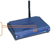
**3.** Verify that the following front panel lights are on: **WLAN** and **LAN**.
