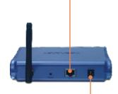
Connect the Power Adapter to the Access Point and then to a power outlet.
