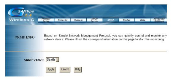
**SNMP:** The SNMP INFO screen allows you to customize the Simple Network Management Protocol (SNMP) settings. SNMP is a popular network monitoring and management protocol.
