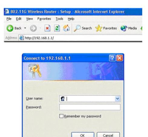
In order to configure the Wireless 11g AP Router, you must input the password into the **Password** box and leave blank on the **User Name** box. The default password is "**admin**".
