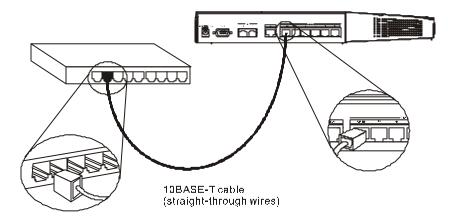
Note that you can connect an end node through the Uplink jack, but to do so you must use a cross-wired cable or cable converter.
