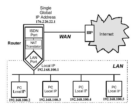
Please note that in the above diagram, the Gateway IP address settings for the local PC's needs to be set to 192.168.100.1, the LAN IP address of the router.
