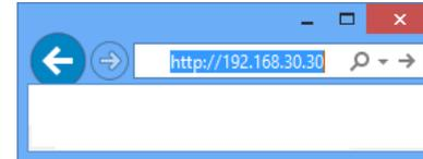
station and connect to it. No password required. Open the web browser on your computer. In the address bar, enter the IP address 192.168.30.30, and then press **Enter**.
