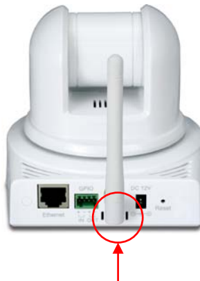
Connecting the External Antenna
