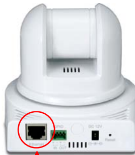
Connecting the Ethernet Cable
