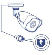
**Power over Ethernet (PoE)** PoE offers cost savings and the flexibility to install this outdoor IR bullet camera up to 100m (328 ft.) from the PoE source equipment.
