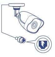
**Power over Ethernet (PoE)** PoE offers cost savings and the flexibility to install this outdoor IR bullet camera up to 100m (328 ft.) from the PoE source equipment.
