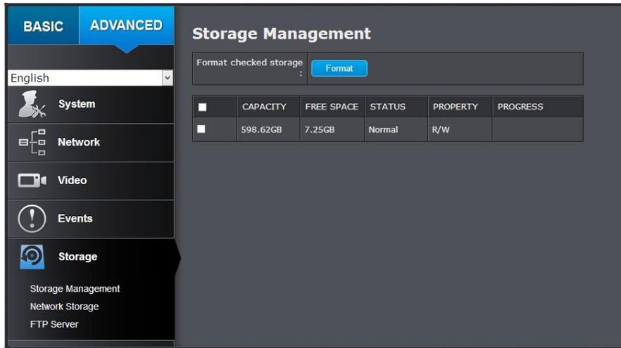
**Format:** Select a network storage volume and then click **Format** to format your network storage. This action will format the network volume (shared folder) for video recording. Placeholder files (formatting files) will be created to make sure disk allocation is appropriate and the file searching is optimized.
