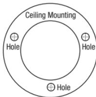
3. Drill holes at each marked position on the template. Make sure the drill bit matches the size of the holes on the template.
