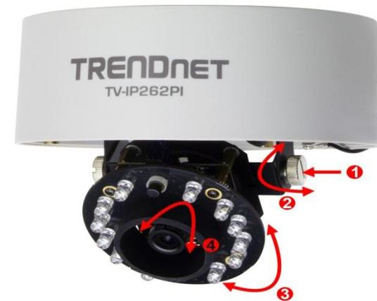
**NOTE:** You can review the image quality from the Web browser when you complete the installation. If the image quality is poor, you have to disassemble the Dome cover to adjust the lens focus until the desired image appears clearly.
