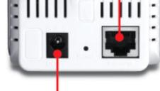
3. Connect the Power Adapter to the IP Camera and then to a power outlet.
