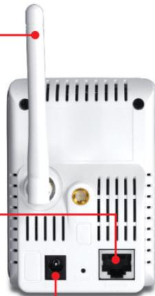
2. Connect a RJ-45 network cable from a Switch/Router to the Ethernet port on the IP Camera.
