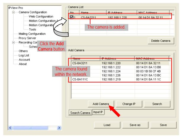
3. Click *Save*, and then click the *System Configuration* button to return to View Window. The selected camera's video will be displayed now. You can click *Save as* to save the selected cameras into the desired path and the selected cameras can be reloaded by *load* button.
