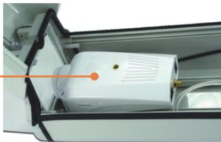
5. Insert the IP Camera's power adapter and Ethernet cable through the mounting bracket.
