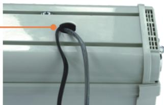
7. Connect the Ethernet cable and power adapter to the camera.
