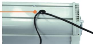
5. Connect the SMA end of the TEW-ASAK(s) to the IP camera.
