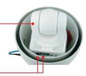
**15.** Connect the network cable and power adapter to the IP Camera.
