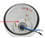
12. Use three round head screws to mount the metal bracket BR004 on top of the 3 Hex screws. The three round head screws are in the plastic bag labeled Q6.
