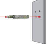
**4.** Align the wall mount bracket with the screws, and then use nuts and washers to secure it.
