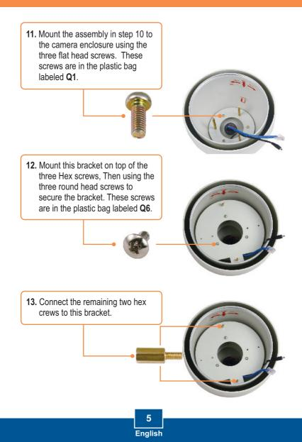
Attach the mounting plate for the camera with 3 small screws. These screws should come with the Internet Camera Server.
