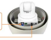
**17.** Place the TV-H400's cover over the camera and rotate the cover clock-wise.
