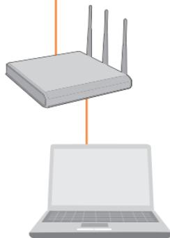
6. Plug a second TPL-302E into an outlet where your remote PC, wireless access point or other device with a built in Ethernet port is located.
