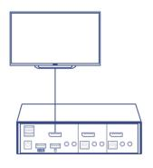
**DisplayPort 1.2**Designed to connect to two DisplayPort computers.
