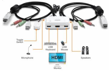
2. Connects the first set of the USB/HDMI/Microphone/Speaker KVM cable into the 1<sup>st</sup> computer and connect the other set of the USB/HDMI/Microphone/Speaker KVM cable into the 2<sup>nd</sup> computer.
