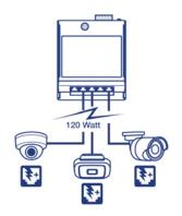
**PoE+ Power** A 120W PoE power budget supplies PoE power from the hardened industrial front access switch to up to five Power over Ethernet devices.
