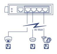
**PoE+ Power** A 90W PoE+ power budget supplies up to four Power over Ethernet devices with PoE+ power.
