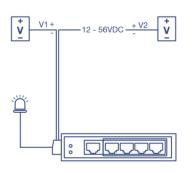
**Fault Tolerance** The industrial Ethernet switch features dual redundant power inputs.
