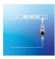
RJ45 Copper SFP Take advantage of unused SFP ports and repurpose them for RJ45 copper gigabit connectivity.
