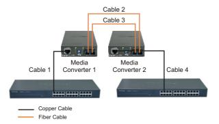
Below are examples on how to read the LLCF Function Table: **Example 1:** If LLCF is enabled on Fiber Converter 1 and disable on Media Converter 2, when Cable 1 link is down, Fiber Converter 1's Copper and Fiber LED and Fiber Converter 2's Fiber LED will shut off. Fiber Converter 2's Copper LED remains on.
