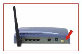
Take the TEW-IA06D connector and connect it to either your Wireless Access Point, Router, or Wireless Card.
