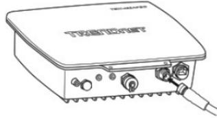
2. Screw-on the other end of the cable connector to the External Antenna. Please tighten both connectors using your fingers. After that, when powering on the Outdoor AP, its wireless signal will automatically go to the External Antenna (bypassing the built-in antenna).
