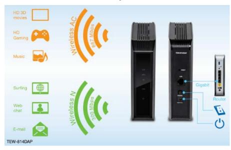
The first access point is installed near your modem/router (typically supplied by your ISP "Internet Service Provider") and physically connected using one of your access point's Ethernet LAN port. The access point is configured to create both 2.4GHz and 5GHz wireless networks your wireless devices (TVs, game consoles, or media bridges)
