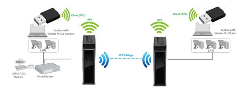
The diagram below illustrates an example of multiple WDS wireless bridge links with access point functionality.
