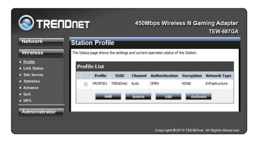
Configure the setting to connect to a wireless network, selection option for network type, SSID, and wireless security. The profile can be edited, deleted and made activated from this option. There are several ways to connect to your wireless network, go through the setup wizard, add a new profile or search using site survey feature.
