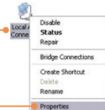
2. Click **Internet Protocol (TCP/IP)** and then click **Properties**. Then click on **Use the following IP address**, and make sure you assign your network adapter an IP address in the subnet of 192.168.10.x.
