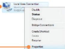
2. Click **Internet Protocol Version 4(TCP/IPv4)** and then click **Properties**. Then click on **Use the following IP address**, and make sure you assign your network adapter an IP address in the subnet of 192.168.10.x.
