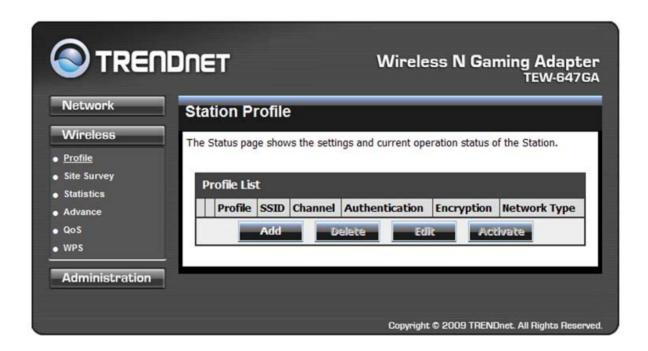
Configure the setting to connect to a wireless network, selection option for network type, SSID, and wireless security. The profile can be edited, deleted and made active from this option. There are several ways to connect to your wireless network, go through the setup wizard, add a new profile or search using site survey feature.
