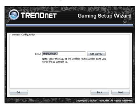
Note: Enter the SSID of the wireless router/access point you would like to connect to.
