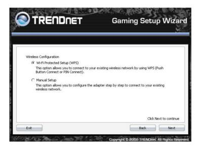
10. You can choose to use **Push Button Method** (PBC) or **PIN Method** to connect to your existing wireless network using WPS type connection.
