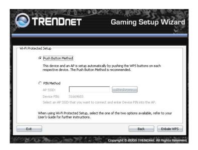
When selecting PBC method, once the **Enable WPS** is clicked, also press the WPS on your wireless router, the devices would negotiate and connection automatically.
