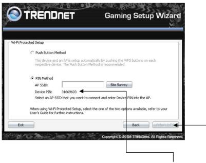
When using the **PIN Method**, please enter the Device PIN number on your router and save it. Use **Site Survey** button to find the router you would like to connect then click **Enable WPS**, then devices would negotiate and connect.
