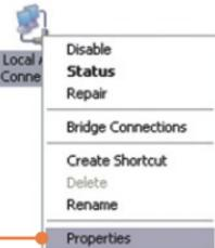
2. Click **Internet Protocol (TCP/IP)** and then click **Properties**. Then click on **Use the following IP address**, and make sure you assign your network adapter an IP address in the subnet of 192.168.1.x.
