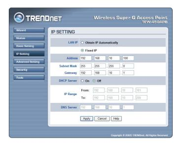
The default IP address of this access point is 192.168.10.100 with the subnet mask of 255.255.255.0. You can type in other values for IP Address, Subnet Mask and Gateway and click "**Apply**" button for the changes to be effective.
