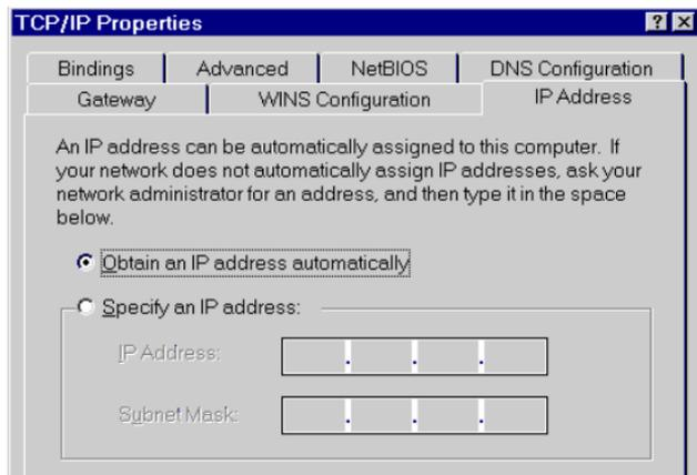
4. "Obtain an IP address automatically" should be selected.
