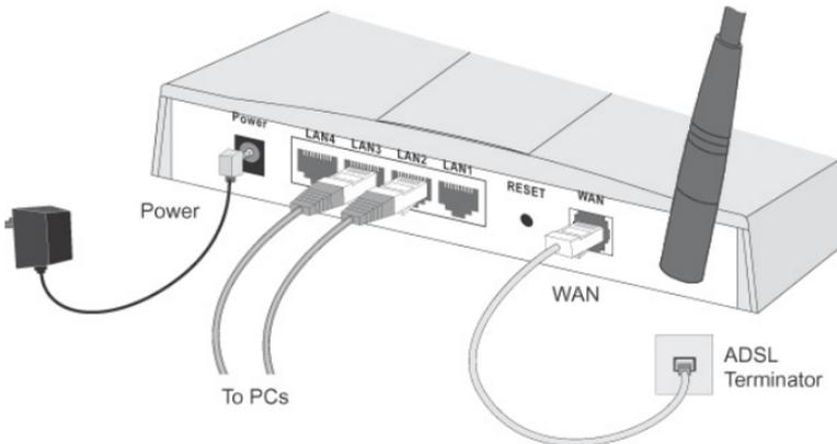
2. Use standard LAN cables to connect PCs to the Switching Hub ports on the TEW-435BRM. Both 10BaseT and 100BaseT connections can be used simultaneously.
