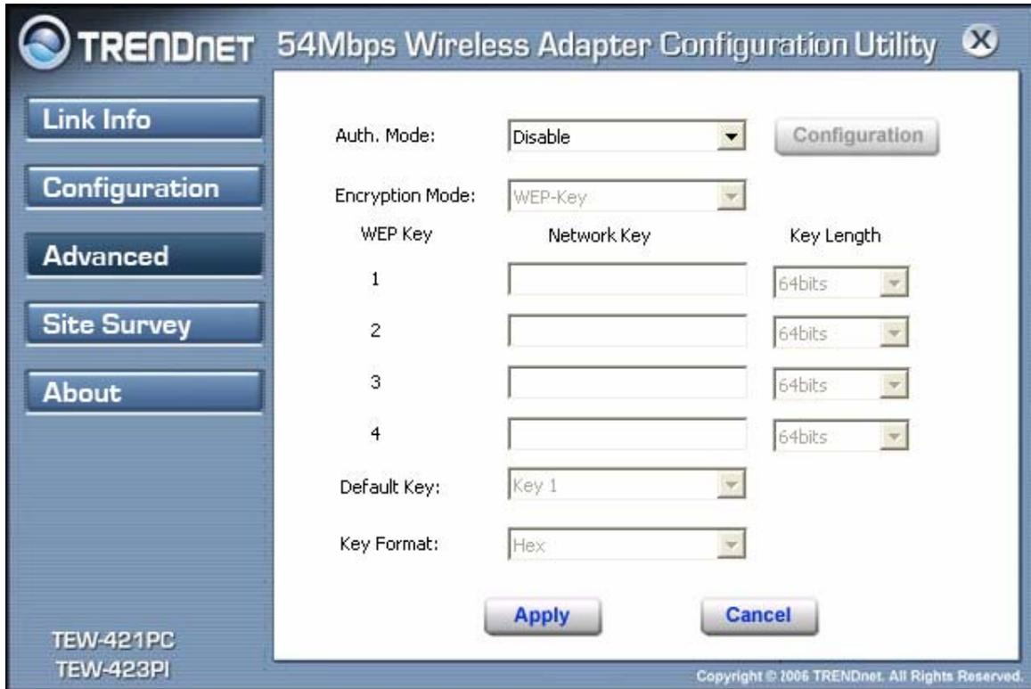
The screenshot shows the 'Advanced' configuration window for the TRENDNET 54Mbps Wireless Adapter. The window title is 'TRENDNET 54Mbps Wireless Adapter Configuration Utility'. On the left, there is a navigation menu with buttons for 'Link Info', 'Configuration', 'Advanced' (which is highlighted), 'Site Survey', and 'About'. The main area contains the following settings:
