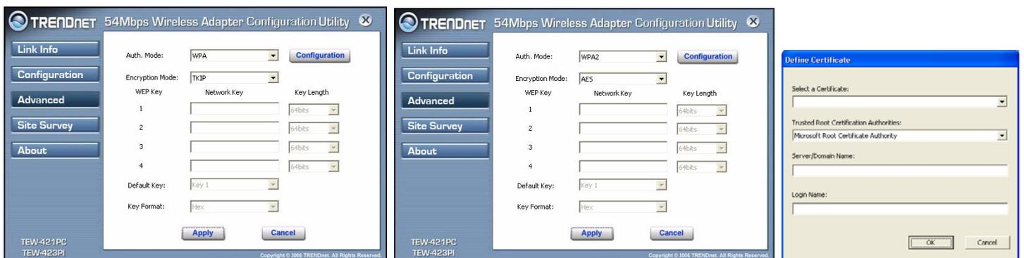
If WPA or WPA2 is selected, the above screen is shown. Please select the encryption type from the drop down menu and press **Configuration** to setup parameters for the RADIUS server.
