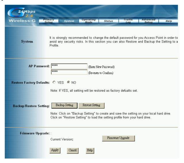
**AP Password:** Changing the password for the AP is as easy as typing the password into the **Enter New Password** field. Then, type it again into the Re-enter to confirm.
