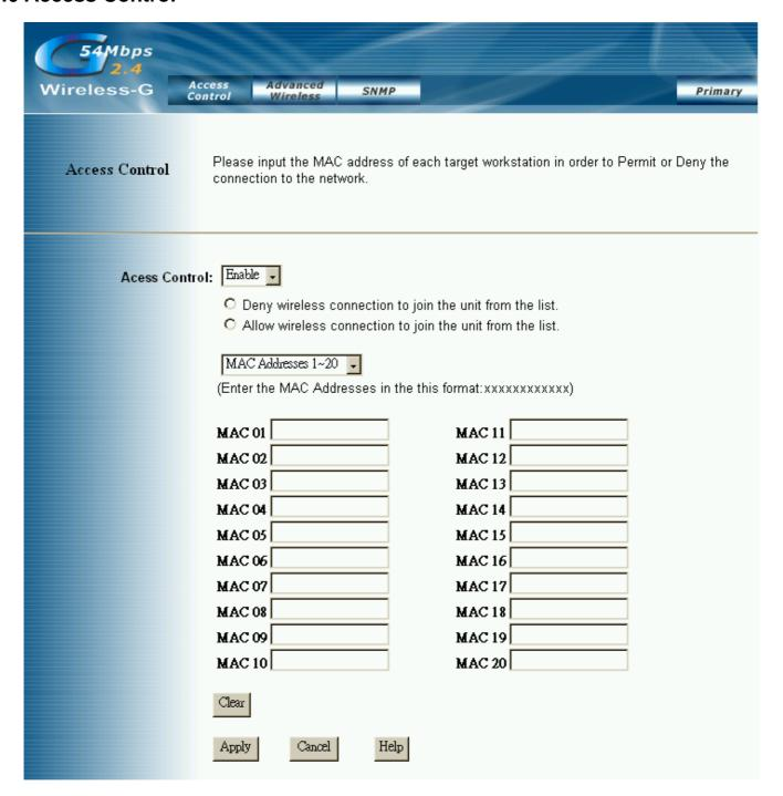
**Access Control:** This function will allow administrator to have access control by enter MAC address of client stations. When **Enable** this function, two new options will show up.
