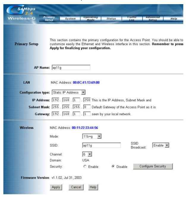
Most users will be able to configure the AP and get it working properly using the settings on this screen.
