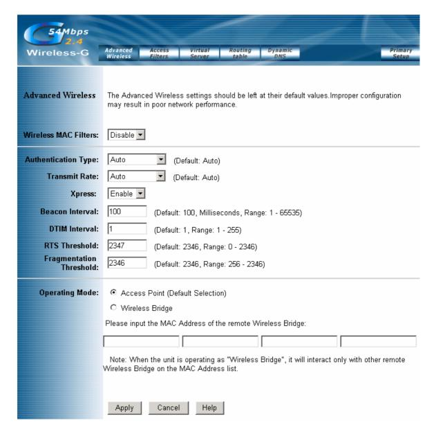
**Wireless MAC Filters:** This function allow administrator to have access control by enter MAC address of client stations. When **Enable** is selected, two new options will show up.
