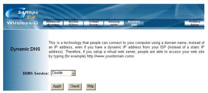
The Router offers a Dynamic Domain Name System (DDNS) feature. DDNS lets you assign a fixed host and domain name to a dynamic Internet IP address. It is useful when you are hosting your own website, FTP server, or other server behind the Router. Before using this feature, you need to sign up for DDNS service with one of two DDNS service providers, DynDNS.org or TZO.
