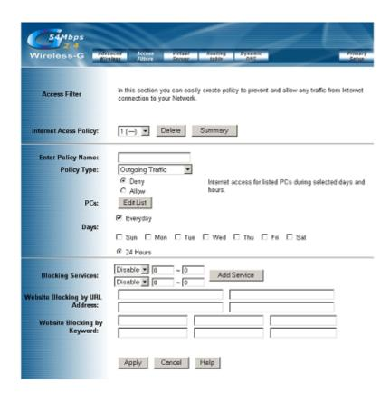
The *Access Filter* screen allows you to block or allow specific kinds of Internet usage. You can set up Internet access policies for specific PCs and set up filters by using network port numbers.
