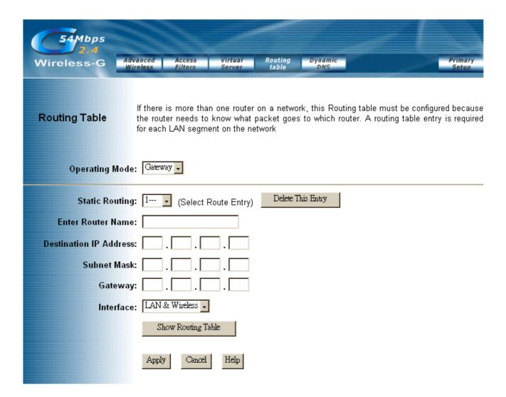
On the *Routing Table* screen, you can set the routing mode and settings of the Router. Gateway mode is recommended for most users.
