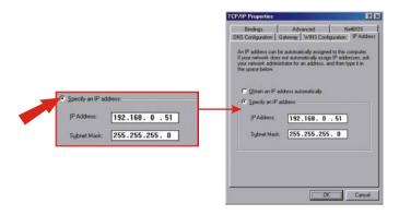
Note: If your network's Wireless Access Point or Wireless Router has a DHCP Server feature, please enable it and configure the wireless adapter to use DHCP IP addresses. After the wireless adapter connects to the Access Point or Router, it will receive addresses automatically.
