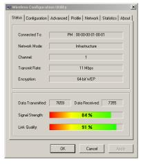
There is another dialog box showing the data transmitted and data received. The two signal lines show the Signal Strength and the Link Quality of the device.
