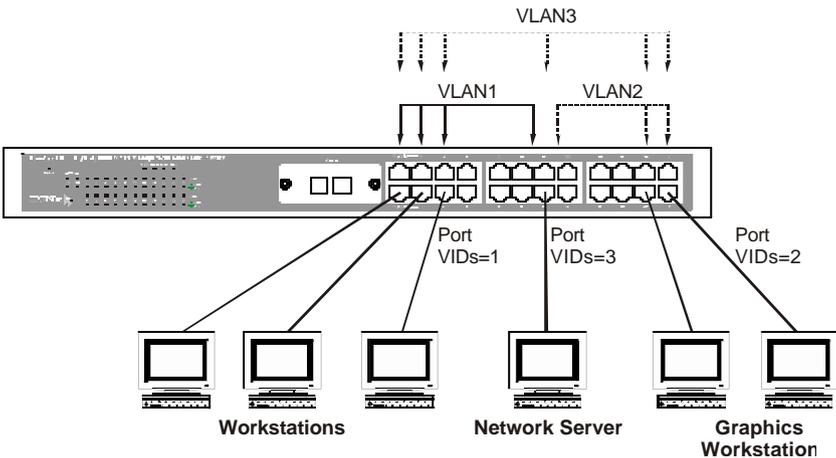
Figure 5-4. Example of typical VLAN configuration
