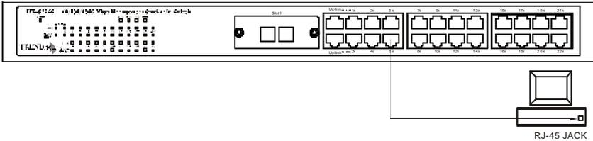
**Figure 4-1. Switch connected to an End Node**
