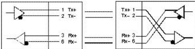
**Figure B-2. Straight cable for Switch (uplink MDI-II port) to switch/Hub or other devices connection**
