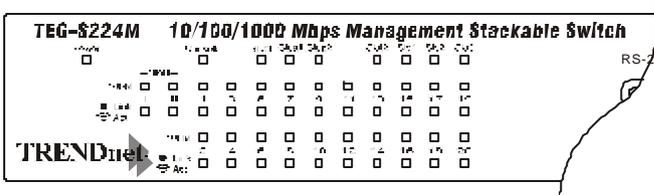
Figure 3-11. The Switch LED indicators
