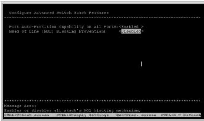
Figure 6-12. Configure Advanced Switch Features screen
