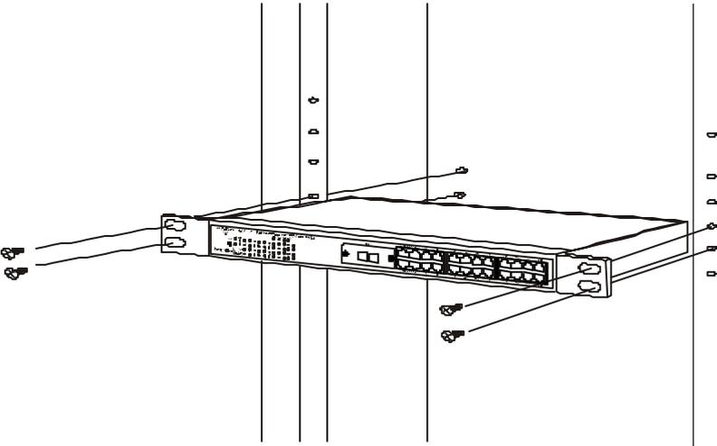
**Figure 2-2B. Installing the Switch in an equipment rack**
