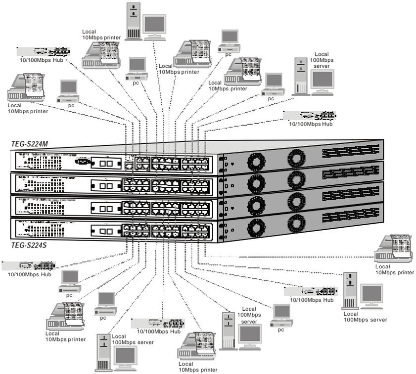
Figure 3-5. Switch stack with example of possible connections
