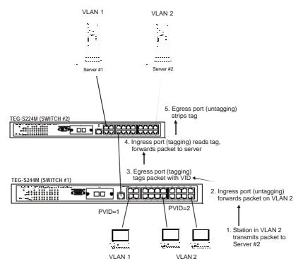
Figure 5-5. Data transmissions between 802.1Q-compliant Switches
