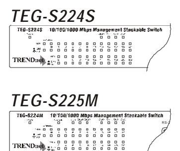
Figure 3-11. The Switch LED indicators
