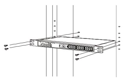
Figure 2-2B. Installing the Switch in an equipment rack
