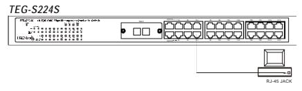
Figure 4-1. Switch connected to an End Node
