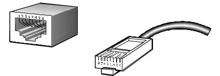
Figure B-1. The standard RJ-45 receptacle/connector
