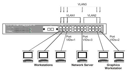
Figure 5-4. Example of typical VLAN configuration
