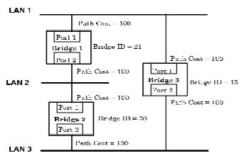
Figure 5-1. Before Applying the STA Rules
