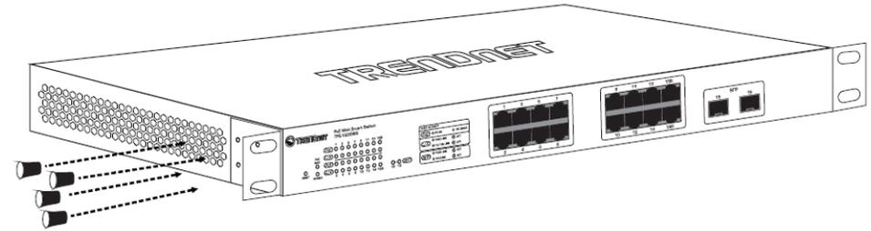
Then, use screws provided with the equipment rack to mount each switch in the rack.
