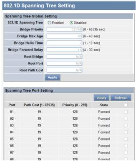
Figure 6. Spanning Tree Setting
