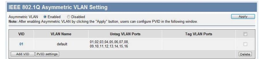
Figure 17. 802.1Q VLAN Setting
