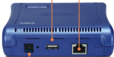
3. Connect the **AC Power Adapter** to the Print Server and then to a power outlet.
